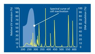
Medium pressure lamps emit a wide-band spectrum, most of which is outside the part of the spectrum that is relevant for disinfection. In addition, the formation of by-products cannot be excluded.
