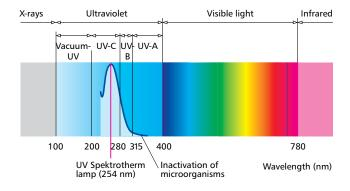
Ultraviolet light is light with very high energy levels and a wavelength of 200 - 400 nm. One of the most effective wavelengths for disinfection is 254 nanometres (nm).
